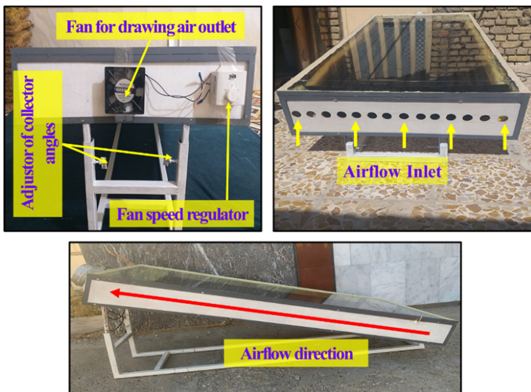
Figure 3. The SAH unit from different directions, highlighting the airflow inlet, outlet fan, and adjustable collector inclination.
