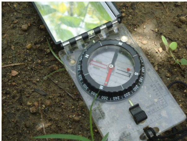
Figure 1. A compass clinometer is employed to fix directional straight-line traverses
