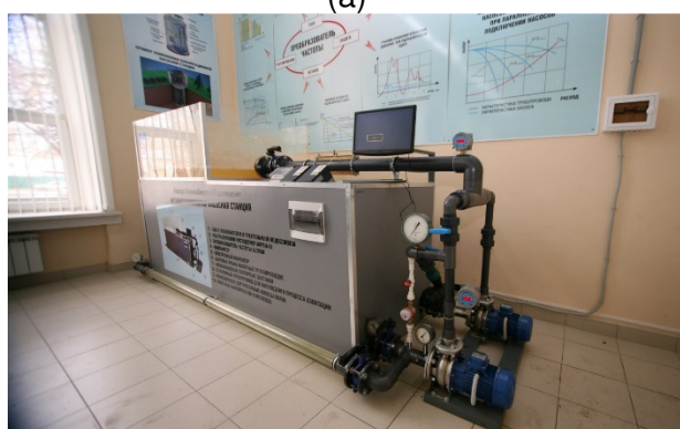
Figure 1. Diagram and general view of the laboratory setup for determining the value of cavitation margin of the volute pumps: 1 – volute pump impeller; 2 – jet device; 3 – inkjet unit; 4 – sensor ultrasonic flow meter; 5, 11, 12, 15 – gate valves; 6 – suction pipe; 7, 9 – vacuum gauges; 8 – flow meter; 10, 13, 14 – pressure gauges; 16 – recirculating line; 17 – pressure tank; 18 – water intake tank; 19 – pressure pipe; 20 – jet device mixer; 21 – piezometer; 22 – sensors ultrasonic flow meter
