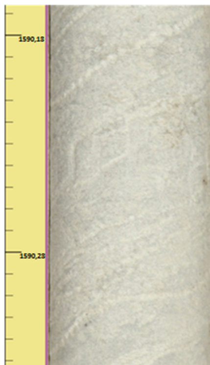
Figure 4. Sandstone with carbonate cement
