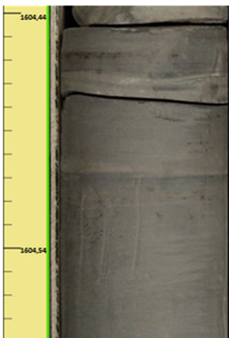
Figure 3. Argillite with a thin-layered texture
