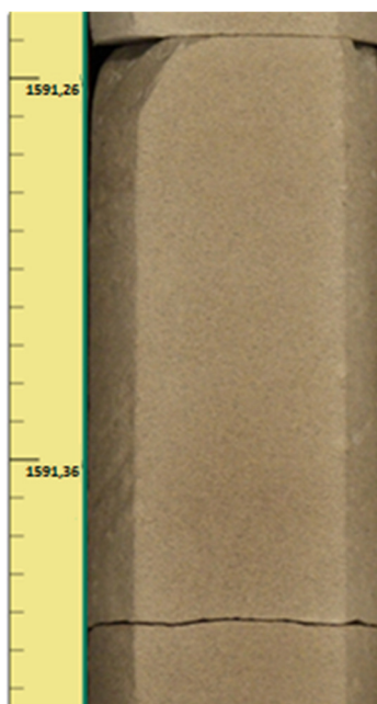
Figure 1. Sandstone fine-grained with scattered clayeyness
