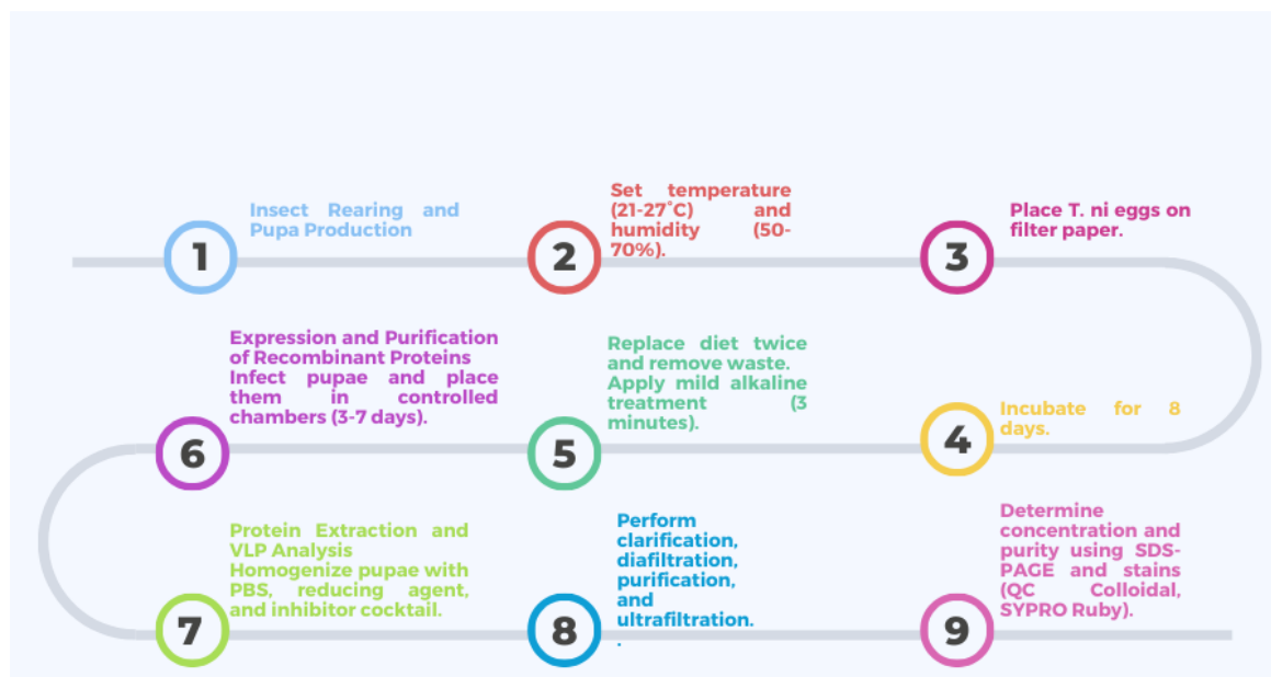
Figure 1. Protein production in the CrisBio system. The figure shows the step-by-step process for protein production using CrisBio technology
